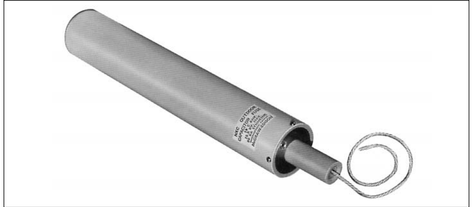
Figure 1. NXC outdoor capacitor fuse, available in voltage ratings of 8.3, 15.5 and 23 kV, offers positive leader wire ejection for reliable interruption and elimination of electrical stress to circuit apparatus. Top end cap has provision for convenient bus bar mounting.
